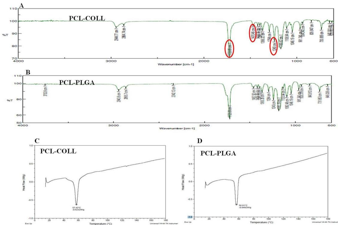
**Figure 2: Characterization of nanofibrous scaffolds. A. FTIR spectra of PCL-collagen highlighting (red circles) amide I, II and III peaks of collagen. B. FTIR spectra of PCL-PLGA nanofibrous scaffold. C & D. DSC curves of PCL-collagen and PCL-PLGA.**
