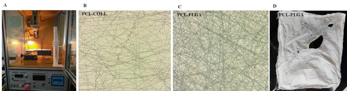
**Figure 1: Morphology of nanofibers. Representative photomicrographs of A. Electrospinning setup B. Nanofibers generated from PCL-Collagen C. Nanofibers generated from PCL-PLGA D. Nanofibrous mat generated from PCL-PLGA.**
